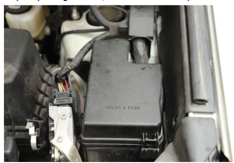
Step 2: check the "circuit diagram" shown on the fuse & relay box cover. There are many kinds of relay inside, we only need the "Start Relay", it's also named as "Start RLY" / "Start" Or just a icon something like half circle with arrow.
