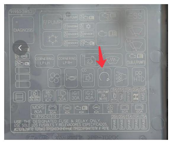
Step 3: according to the "circuit diagram" to find out the right relay at the right location.
