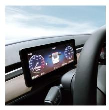
18 If the screen can not light up, but the original screen is bright, check the screen power cable whether is connected. If the original screen is not bright, then get off the car, turn off the engine, and lock the car, wait for 1 minute, then restart the car. If the screen still can not activate, then press the two buttons of the steel wheel for a minute or so, and the screen will restart.
