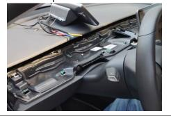
Count from the first hole, and count to the 20th grid, which corresponds to the first pin of the screen base, and the red power supply corresponds to the 22nd hole (then marked on the 20th grid)
