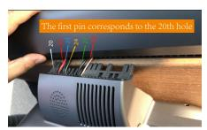
The base here must be pressed to the bottom, make sure to insert the buckles in parallel when installing, if not pressed to the bottom, the screen may shake up and down after tightening the screws.
