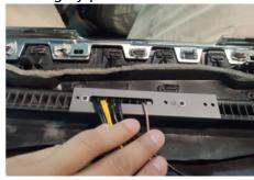
After fixing the plate, insert the plugs corresponding to all colors, Note: Please connect the plug on the arrow position, be sure it had connect tight. And use the gaffer tape to further tight the plug connect position (like the picture) to avoid any problem caused by the plug became loose during usage process.
