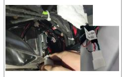
6 Insert the connected plug into the original position of the OBD plug
