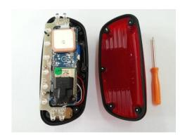
a. Unscrew device. (For T18 and T18H, please unscrew the SIM slot cover instead of the front cover)
