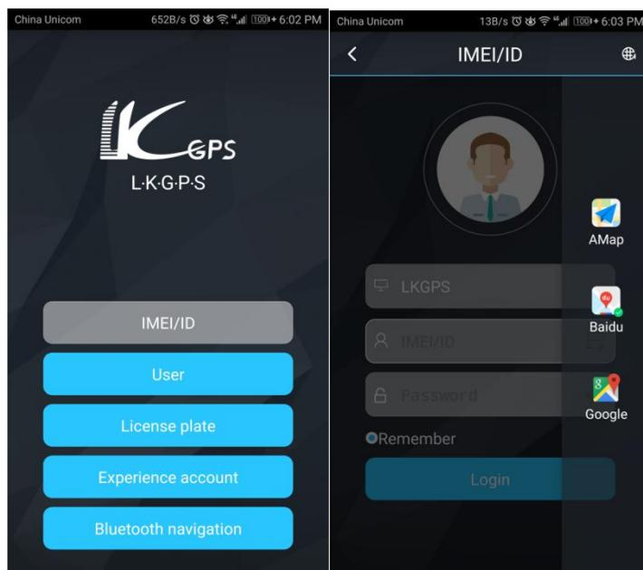
8.2.2 Select "IMEI / ID login" for the first login, select "666" for the first column of address, input 10 digits on the device barcode, and the default password is 123456, Click "log in" to log in
