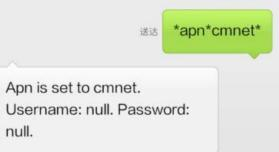
C. Your cellphone will receive SMS reply, says the appointed APN is set (See screenshot as below). Notes:! 1. No matter what APN settings you send to the device, system will reply reply as what you set. But it doesn't mean the device has connected to server successfully. You have to finish the second step to make sure the APN settings is correct.!
